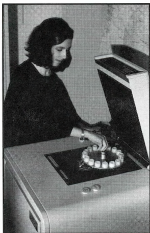
Geochemical analysis of artifacts using X-ray fluorescence.
