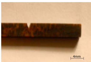
Figure 2.3: Samples prepared for Single edge V notch beam
