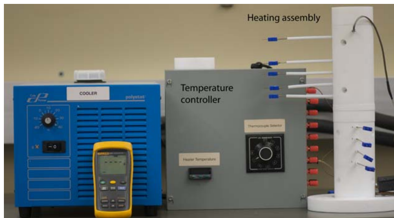
Figure 2.4: Axial heat flow setup for measuring room temperature thermal conductivity [30].
