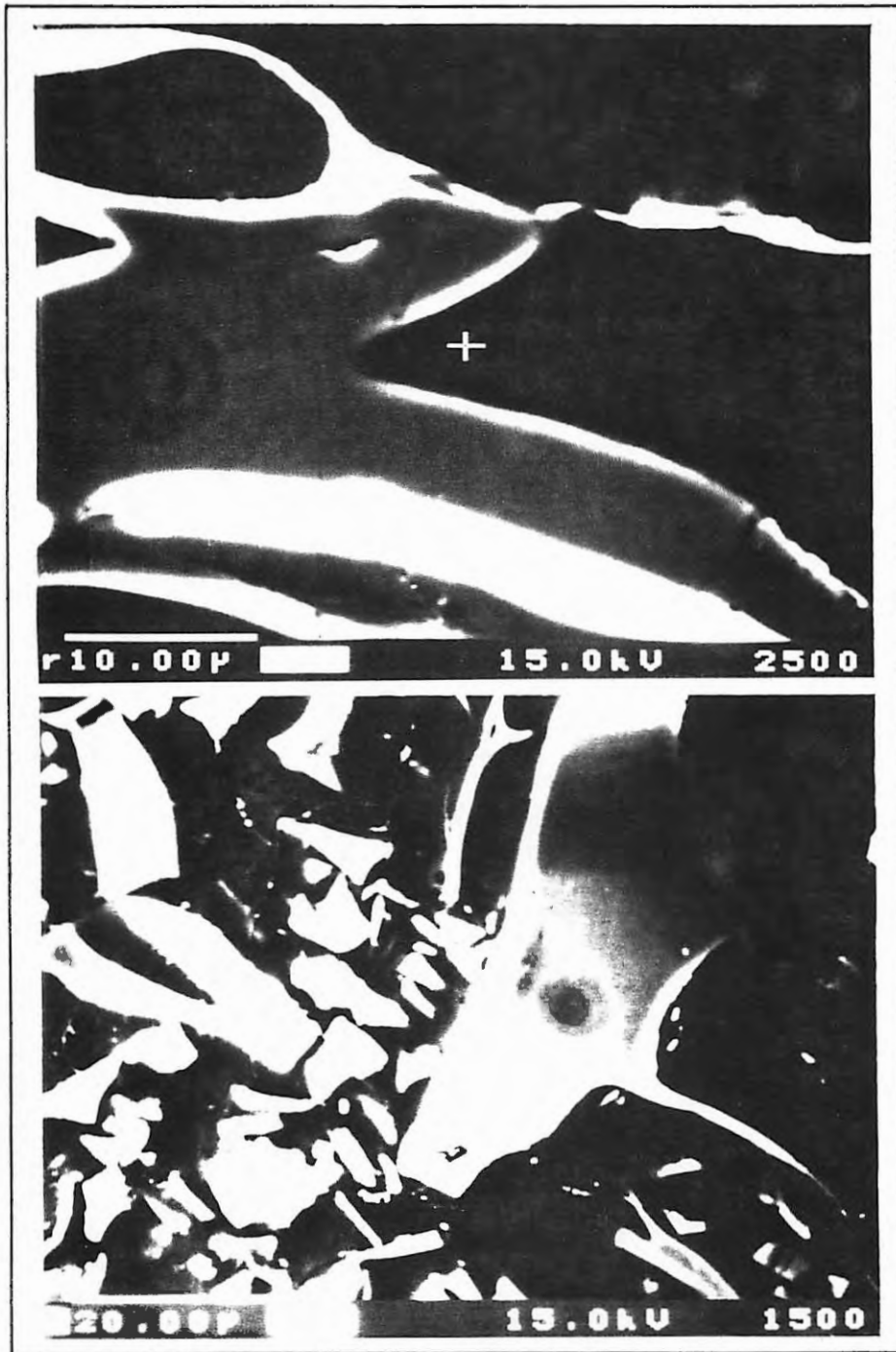
Plates 24 and 25. Top (24): SEM of elongate tephra shard from a lapillus originating from Crater Lake (MAZA-9); 2500x. The circular feature on the smooth flat surface of the shard in the left-hand side of the image is the damage scar left by the electron beam after the glass was analyzed with the electron microprobe. The dark oval structure above the scar is a small vesicle. Bottom (25): SEM of a platy tephra shard from the Rock Mesa eruptions (ROCKM-4); 1500x.
