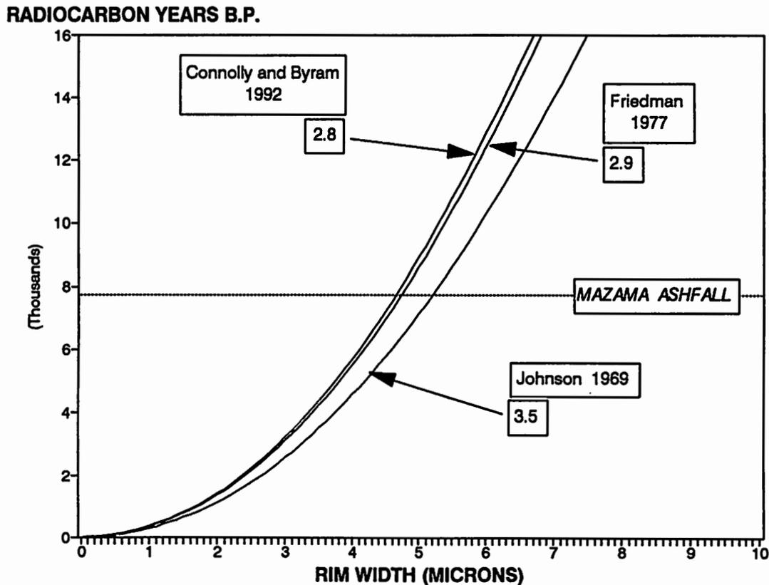
Figure 5-9 Published and proposed obsidian hydration rates for selected sources. (The numbers refer to rates in  $\mu\text{m}^2/1,000$  years, e.g.,  $2.9 \mu\text{m}^2/1,000$  years).
