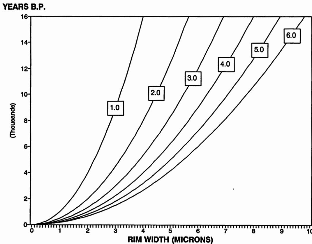
Figure 5-3 Examples of the results of different hydration rates applied to the diffusion model ( $x^2=kt$ ) of hydration developed by Friedman and his associates. (1.0 = rate of  $1 \mu\text{m}^2 / 1,000$  years, and so on).
