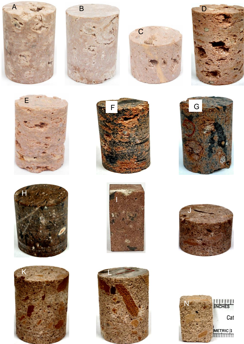
Figure 12. Photo of the samples used to determine porosity for various locations within the RSPT (powdered samples O and P not shown). Cylindrical samples measure approximately 1 inch (25mm) in diameter. Samples I and N are cuboid shaped.
