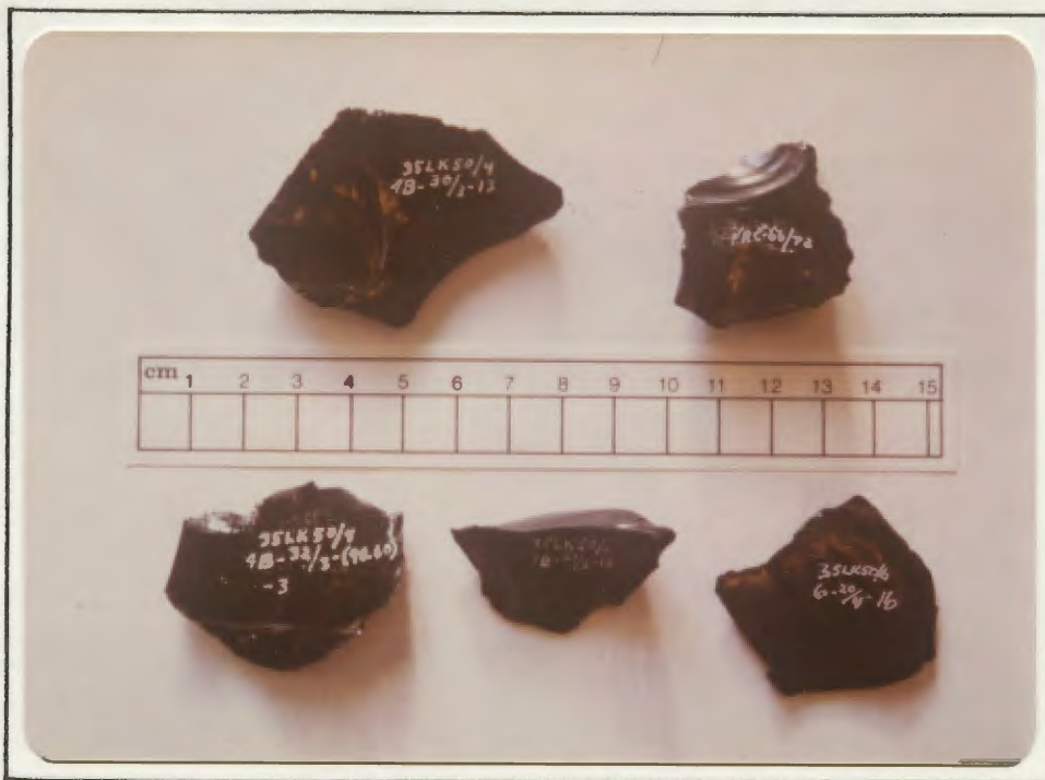
Plate IX-4: Obsidian artifacts from Fort Rock Cave and the Connley Caves prior to their preparation for X-ray fluorescence analysis and thin-section examination.
