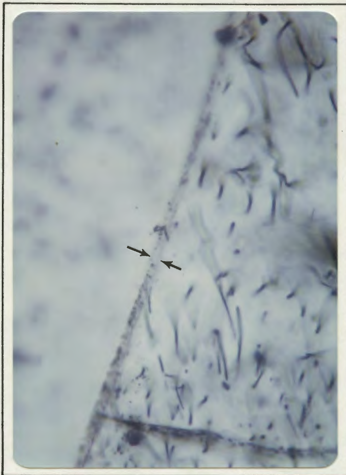
Plate 11: Photomicrograph of a hydration rim that has formed on the surface of an obsidian artifact. The width of the rim pictured is about 6 microns. Nicols not crossed, x150. The obsidian artifact occupies the right half of the photograph.
