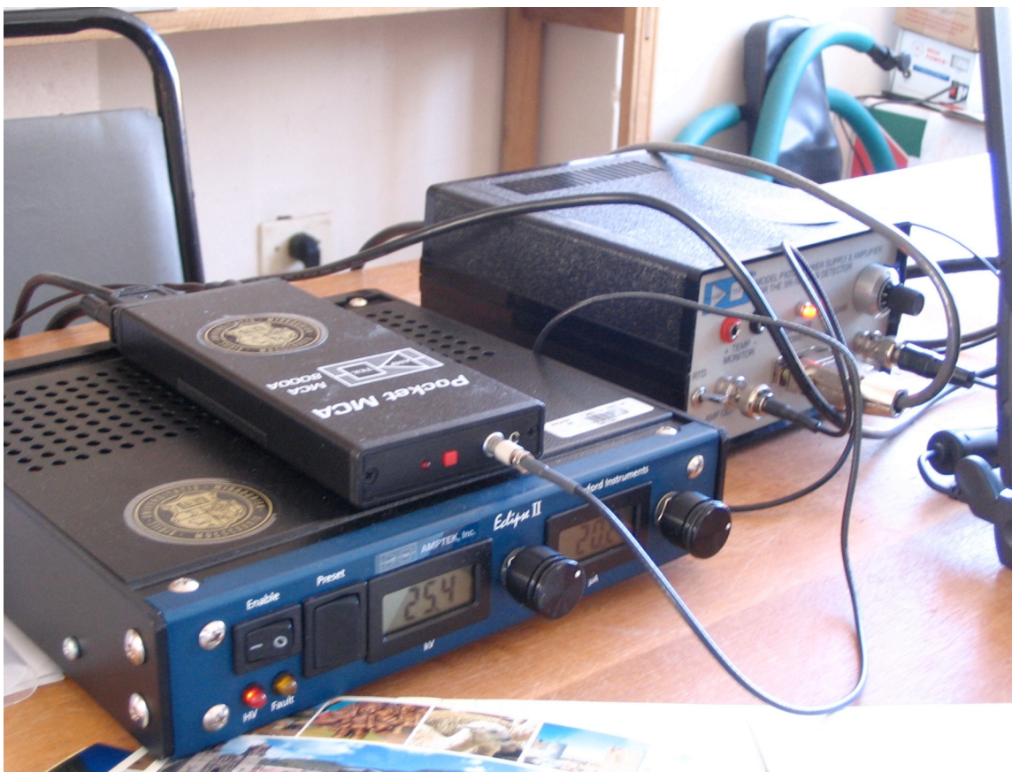
Figure 5.3: X-ray and detector power sources and multi-channel analyzer (MCA)
