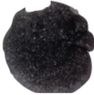
Figure III.15: Obsidian after thermal annealing at 900°C
