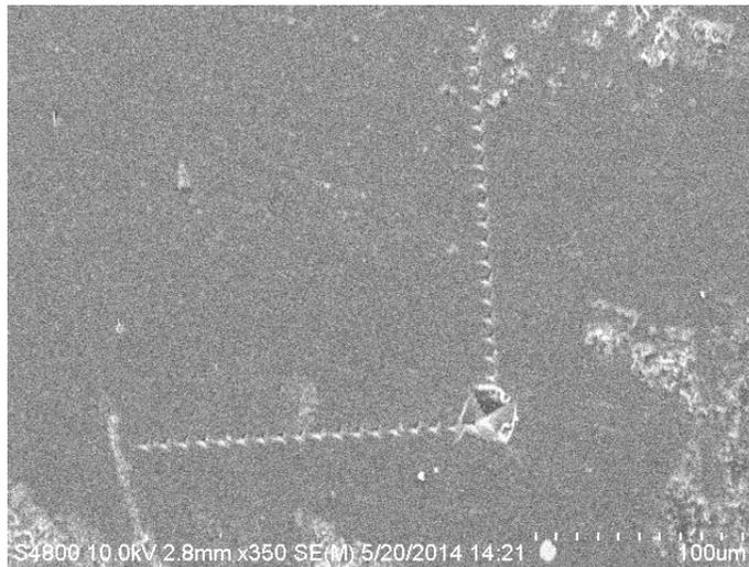
Figure III.19: SEM: Nanoindentations around vickers Indent
