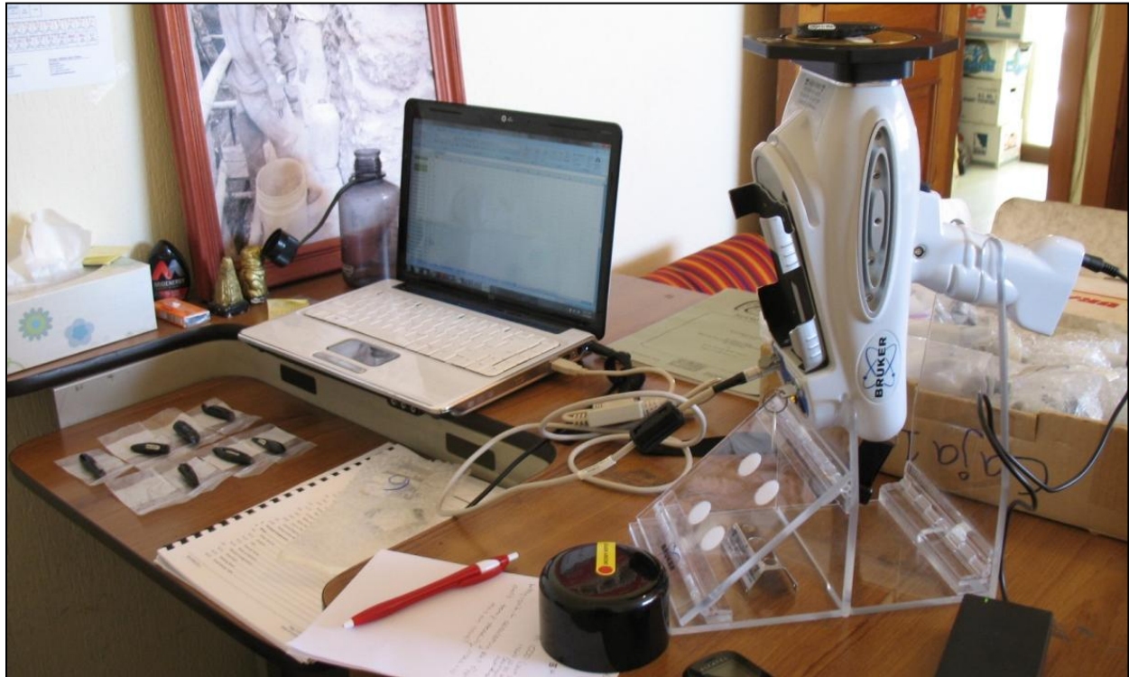
Figure 5. The Bruker Tracer III-SD T3S1995 PXRF set up for testing in the FARES laboratory.
