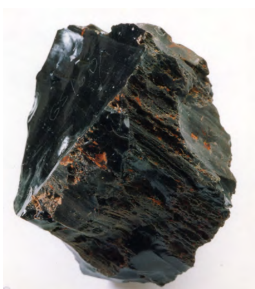
Figure 4.15: Photograph of a sample showing the correspondence between corrosion rates and flow banding
