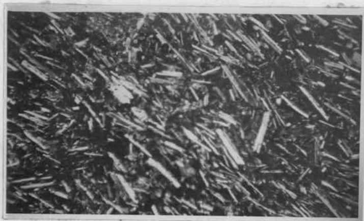
Fig. 16. Photomicrograph of specimen B-193. Exhibits a trachytic texture. Nicols crossed, 32 X.
