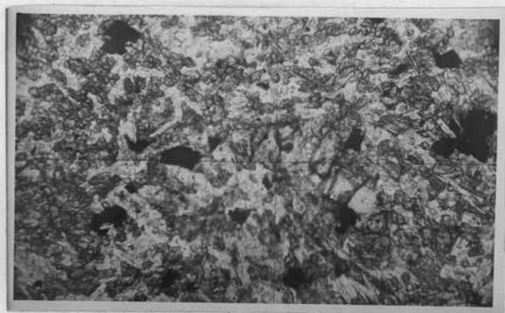
Fig. 21. Photomicrograph of Intercanyon basalt, sample L-83. The texture is diabasic and the minerals shown are olivine, augite, magnetite, and plagioclase. Nicols crossed, 32 X.
