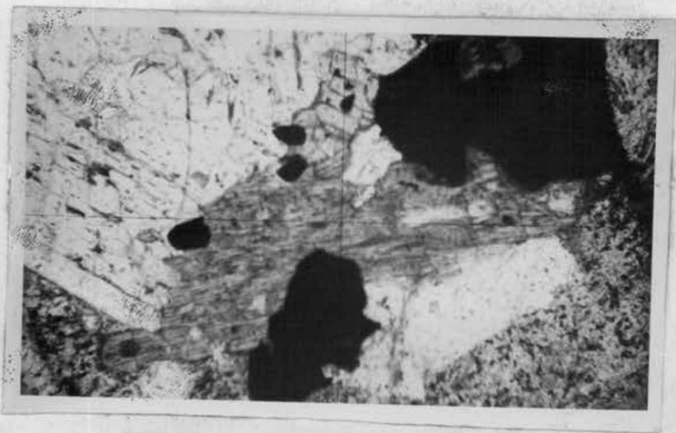
Fig. 13. Photomicrograph of the same basalt sample. Crystals are hornblende, magnetite, plagioclase, and augite. Plane polarized light, magnification 32 X.
