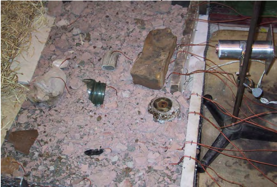
Figure 4.3: Sediment bed with artifacts, thermocouples, and radiometers.
