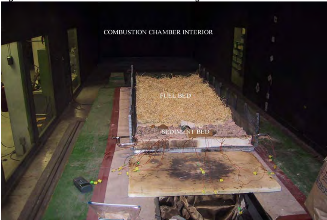
Figure 4.2: Interior of Combustion Chamber showing burn table.
