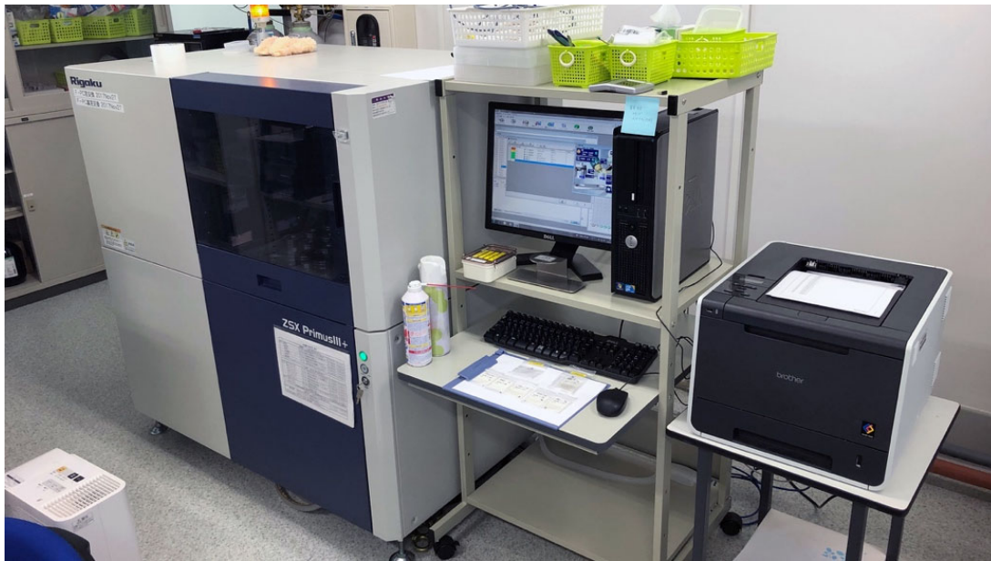
Figure 6. WDXRF instrument (Rigaku Primus III+) installed at Meiji University (Center for Obsidian and Lithic Studies, Nagano).
