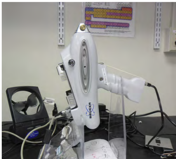
Figure 2. Portable EDXRF Bruker Tracer III - Sitting vertically to optimize the analysis (photo by Julien Pessarossi-Langlois). Missouri University Research Reactor Laboratory.
